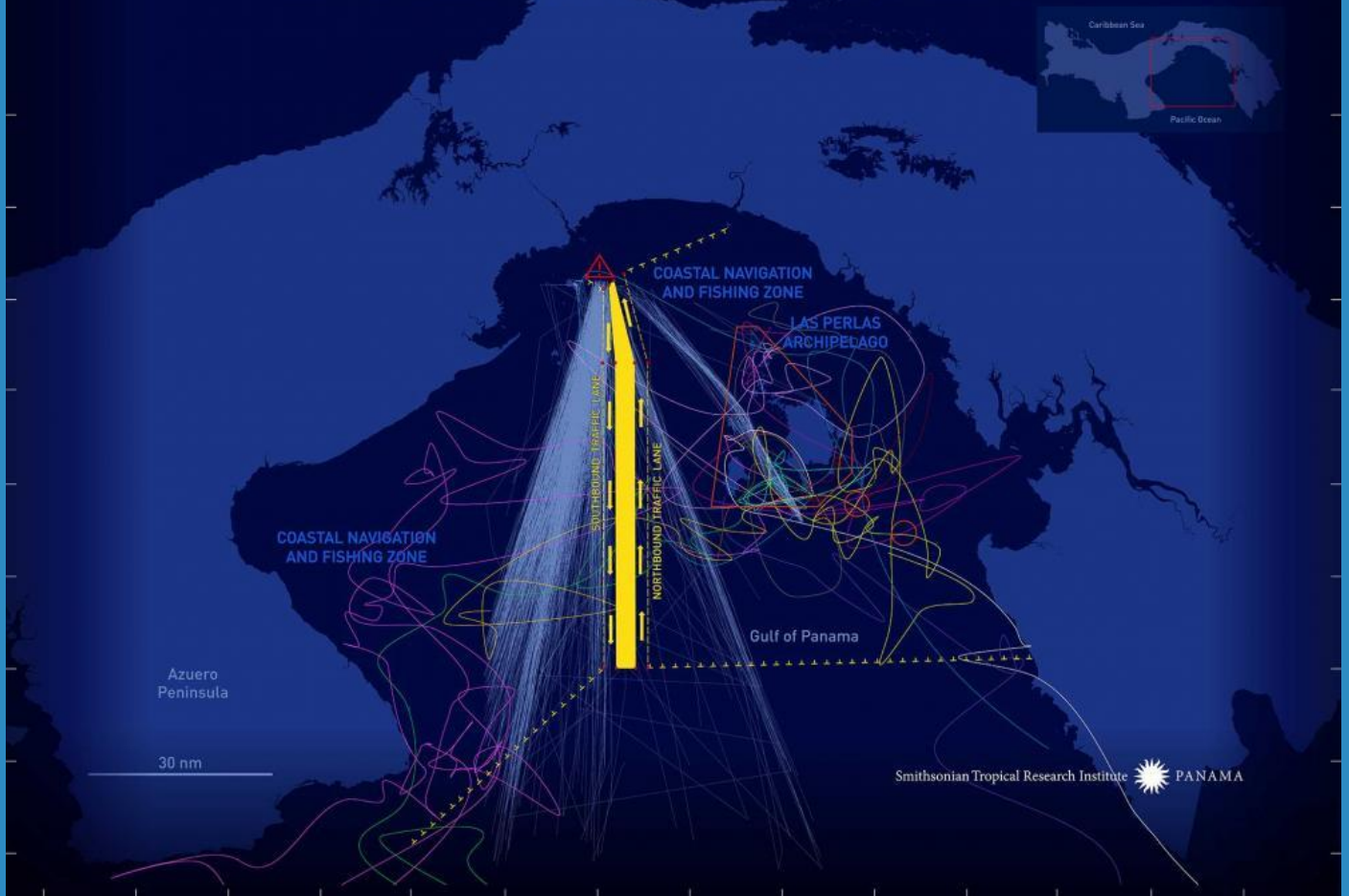
Figure 4: Traffic Separation Scheme, approved by the Republic of Panama and adopted by the International Maritime Organization, used by Panama Canal Authority, the Panamanian shipping lanes were implemented since December 2014. Reproduced from Smithsonian, Science & Conservation (2016).
